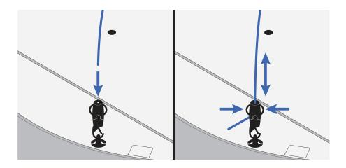
Gripple working load limit at vertical: 33 lbs (15 kg)
