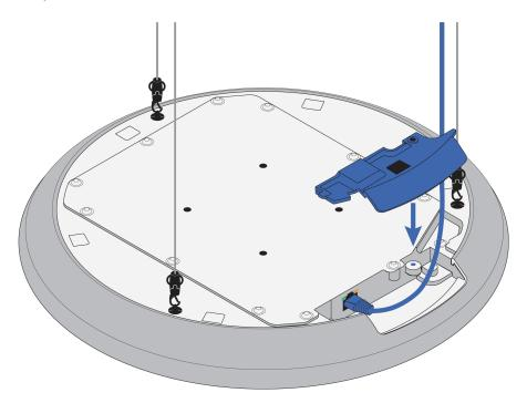
7. Attach the back cover. The cover's 6 clips snap into the 6 square holes on the microphone.
