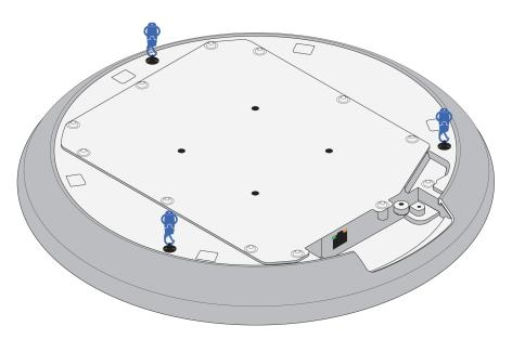
3. Thread the included steel cable through the connectors as shown. Squeeze the sides of the connector to adjust the cable's length.
