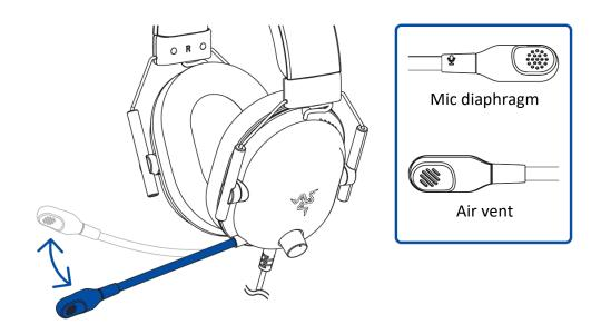
The recommended mic-to-mouth distance for optimal sound capture is 1.5 cm to 3 cm (0.59 in to 1.18 in).
