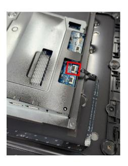
S13 Tear off "MYLAR USB board" from "Main Shielding"
