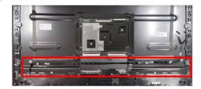
S20 Disassemble "Middle Frame" from "ASSY CHIN" and "Panel"
