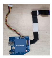
S15 Remove a "GASKET" from the "USB board"
