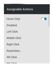
Of particular note is the "Hover Click" option, which enables the user to execute the action with the pen tip hovering near the screen instead of directly touching it.
