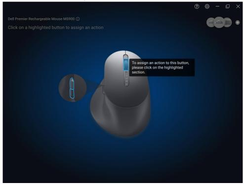
To assign an action, click on a highlighted button or key. The "Assignable Actions" box provides a list of selectable actions.
