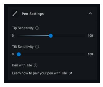
For supported applications such as Microsoft Whiteboard, the sensitivity settings will vary the brush width based on the amount of pressure and angle of the pen tip applied to the screen.
