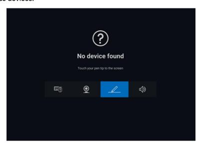
After selecting the appropriate icon, pressing the pen tip to the screen will activate a special pop-up window to allow pairing of the device.
