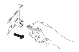
2. Pull down the latch and remove the module.
