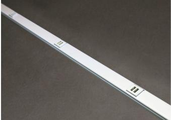
5' (1.5m) length with 12" spacing. USB is 2.4 Amps (shared between two ports) 5VDC. .040" (1.0mm) steel housing. Packed two per carton. Each unit supplied with one (1) Coupling and two (2) Blank End Fittings. Each USB module provides 2 ports with 2.4 Amps of shared charging. Please note the charging load on one module will not affect the charging performance of the other USB modules in the product.
