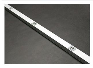
Available in 5' (1.5m) length with 12'' spacing. USB is 2.4 Amps (shared between two ports) 5VDC. .040'' (1.0mm) aluminum housing. Packed two per carton. Each unit supplied with one (1) Coupling and two (2) Blank End Fittings.
