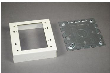
For standard shallow switches and receptacles including single-gang combination devices. Base has two 1/2" trade size KOs. Larger gang boxes available by special order. Two-gang: 4 3/4" L x 4 3/4" W (121mm x 121mm). Accepts NEMA double-gang standard faceplates. NOTE: Certified to Canadian Safety Standards for sale in Canada. When ordering these products, change the "V" color prefix to "vc" or the "WH" color suffix to "WHC" to denote the Canadian versions.
