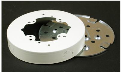
Cover accepts fan bracket device with mounting centers of 3 3/16" (81mm). Base has six mounting holes and 4 1/2" trade size KOs. #10 mounting studs provided. Rated for fans and fixtures up to 50 lbs. NOTE: Certified to Canadian Safety Standards for sale in Canada. When ordering these products, change the "V" color prefix to "vc" or the "WH" color suffix to "WHC" to denote the Canadian versions.
