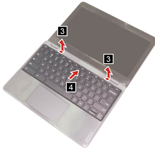
Figure 7. Open the keyboard sockets and lift the keyboard
