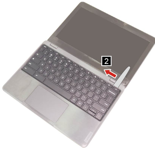
Figure 6. Use the pry tool to pry up the top right corner of the keyboard and slide it to the left
