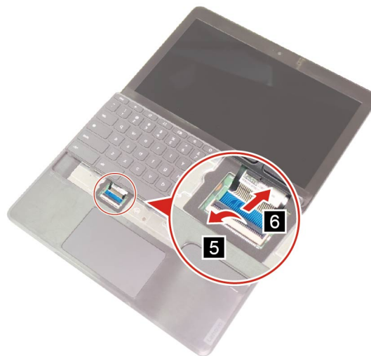
Figure 8. Disconnect the keyboard cable
