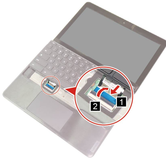
Figure 9. Connect the keyboard cable
