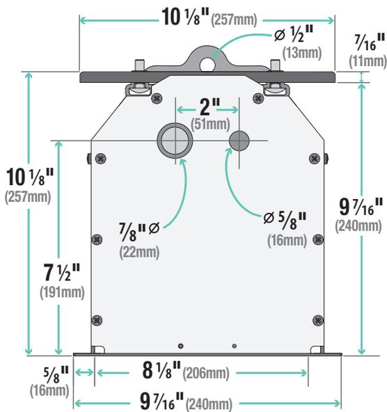
Standard Motor Wiring is on the AUDIENCE LEFT END of Screen Case.
