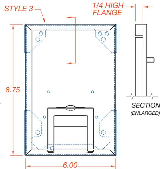
**\*\*Note:** Cover Shim Kit (FL-200-CSK) may be required to set the height of box "Pre-Pour" so the top of Finish Cover matches top of finished floor.
