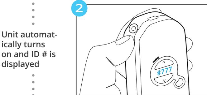
Unit automatically turns on and ID # is displayed
