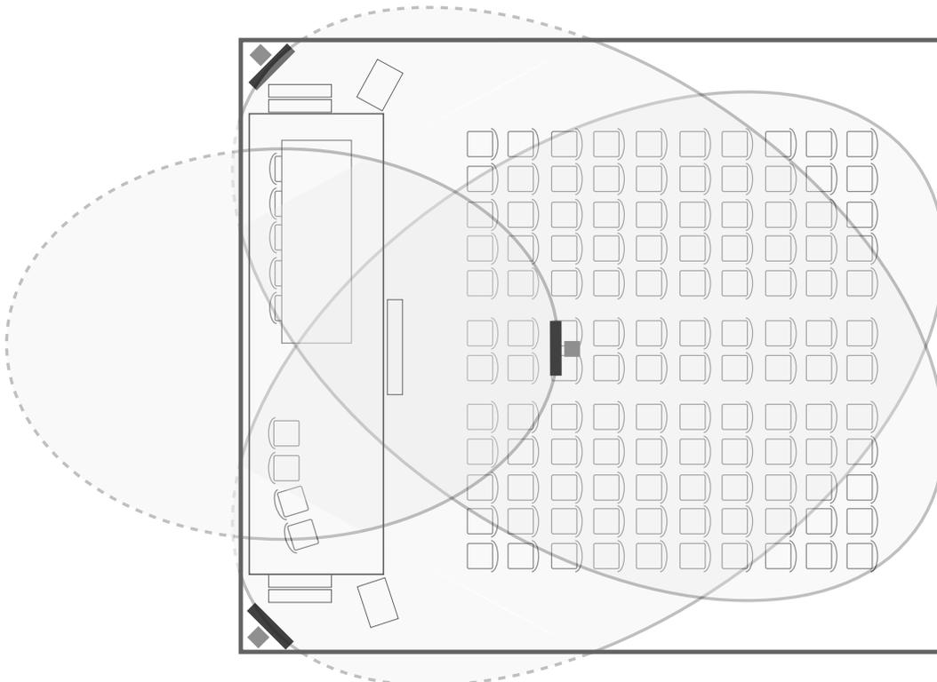
*Except in small rooms, it is recommended that at least two radiators are used to prevent shading of the IR signal.*
