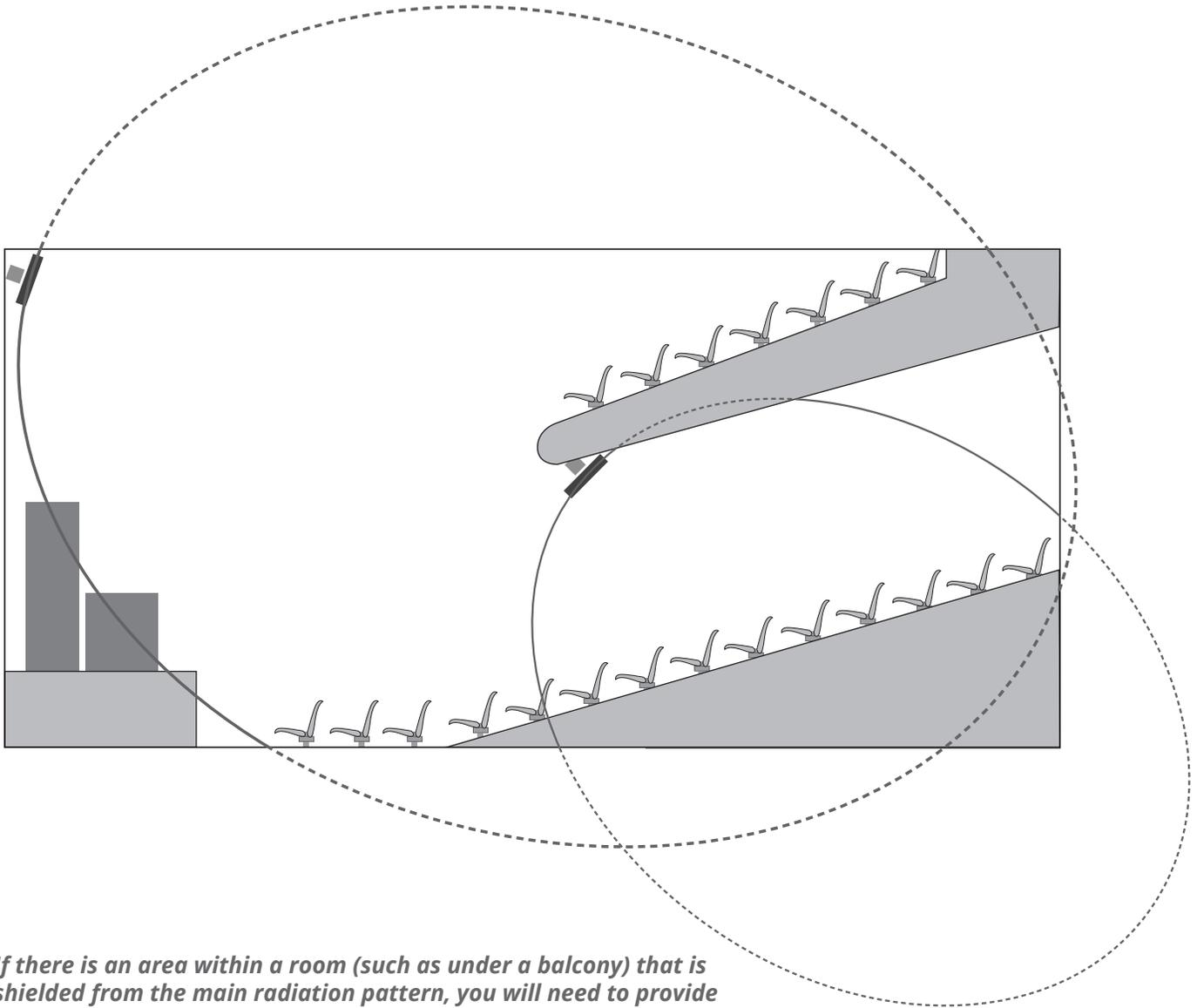
*If there is an area within a room (such as under a balcony) that is shielded from the main radiation pattern, you will need to provide additional radiator(s) to cover this area.*
