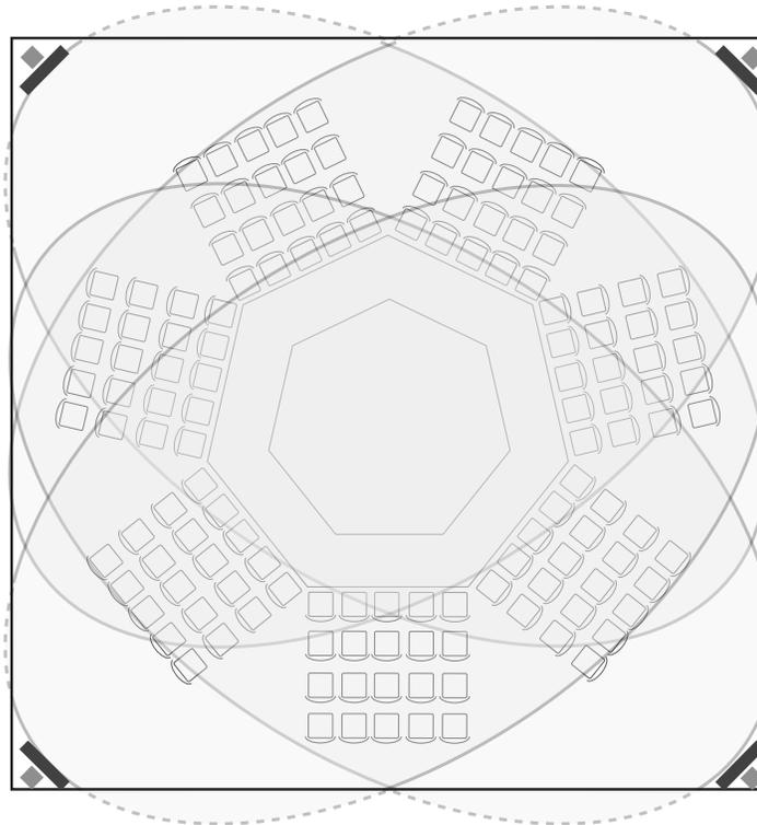
*In this example a total of four radiators, one in each corner, ensures good coverage at all locations and orientations.*
