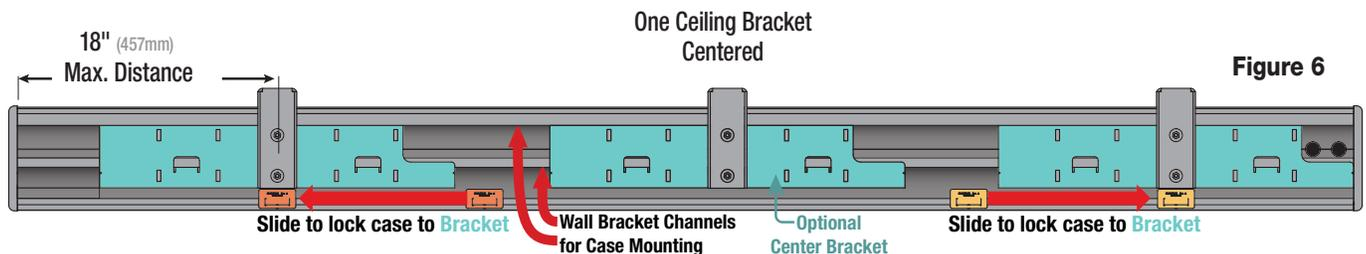
6. Once the case is settled on the mounting brackets, slide the Bracket Locks to the center of each mounting bracket (see Fig. 6) and secure set screw on the lock.
