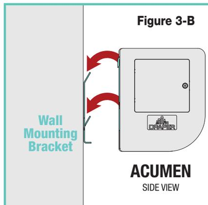
4. Holding the case by the endcaps, lift it up and over the cleats on the **mounting brackets** (see Fig. 3). **Wall Bracket Mounting Channels** are shown in Fig. 4 below.
