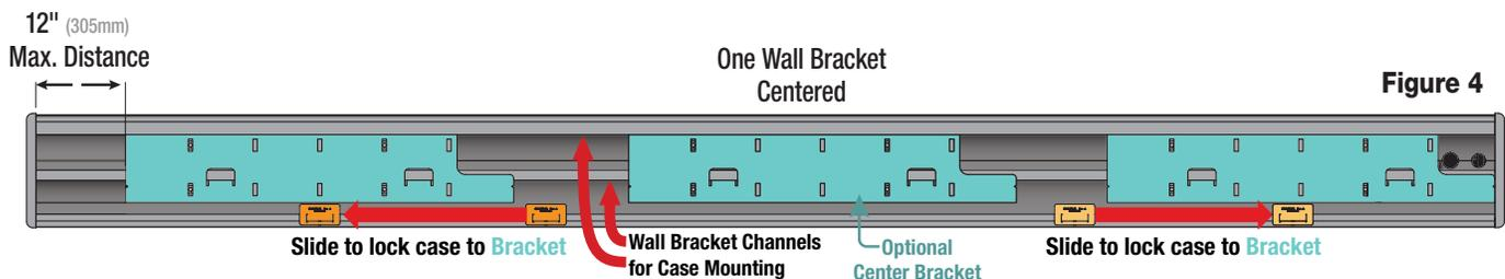
5. Once the case is settled on the mounting brackets, slide the **Bracket Locks** to the center of each **mounting bracket** (see Fig. 4) and secure set screw on the lock.
