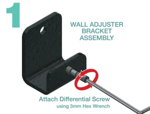
2. Attach two (2) Wall Adjuster Brackets to the back side using a 3mm hex wrench.
