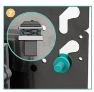
**Spring loaded mounting studs** push cabinets into the final Z-axis position.
