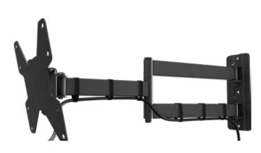
Articulating mount for 13" to 49" displays. Multiple joint arm holds display 1.9" from wall when retracted and 21" when fully extended. Smooth tilt adjustments of  $\pm 10^\circ$  (forward) and  $\pm 10^\circ$  (back) and 3° side-to-side roll facilitates a variety of viewing angles and perfect positioning. Three attachment points for wood studs and concrete walls provide additional security. Optional cable management for clean look.
