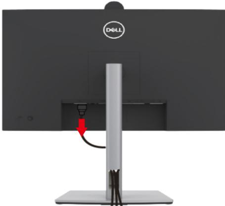
**S3** Remove stand from the product.(Press the stand release button, lift the stand up and away from the monitor)
