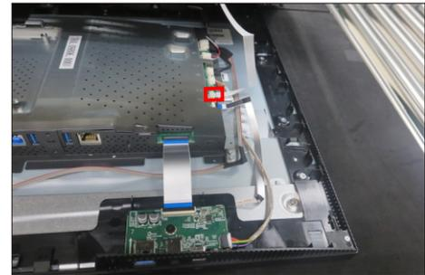
Use a Philips-head screwdriver to remove 3pcs screw for unlocking the joystick board, and then tear off all the tapes on the back of the cable and release the joystick cable from the rear cover.
