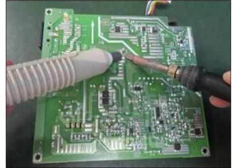
S24-5 Lift the bulk cap. up and away from the PCB.
