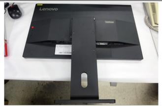
Remove 4pcs screws for remove the stand base
