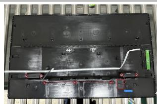
Tear off all tape, and release the key board by removing 2pcs screws
