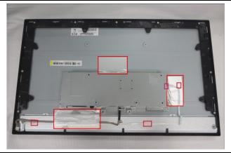
Disconnect the LVDS cable and panel lamp cable. Lift up the bracket and put it aside Remove all screws for unlocking middle bezel. Tool: Screwdriver #2 Disassemble the middle bezel with the panel module Release the keypad PCB from the middle frame
