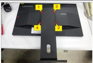
Use the C/D disassembly tool to release rear cover hook from disassemble hole on bottom
