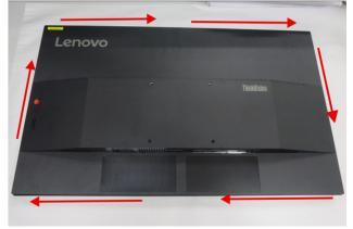
Lift the rear cover up, then disconnect the function key cable and speaker cable, and then remove the rear cover
