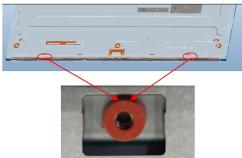
**S20** Unlock 10 PCBA screws to disassemble I/F BD, SPS BD and LED Driver BD from Main SHD
