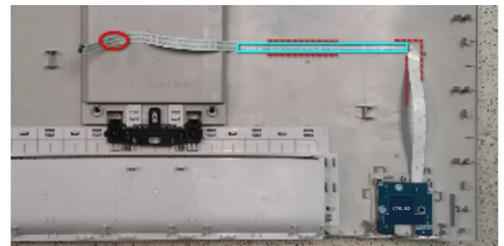
**S6** Unlock screw\*3 to disassemble CTRL BD from Rear Cover
