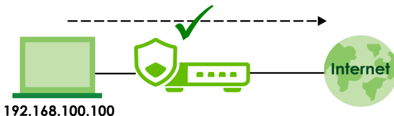
Figure 249 IP Exception Bypass Source Example
