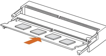
2. Push down until the modules snap into place.
