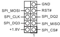
This ROM Recovery Connector allows qualified technicians to reload firmware into the SPI boot flash in case there is problem with the data.
