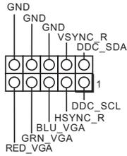
This VGA Connector provides VGA interface for your monitor.
