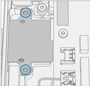
2. **Connect Micro SD FPC** – Making sure tweeter connector is out of the way, align the Micro SD Slot connector with the motherboard and press in firmly. A small click may be heard.
