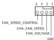
This motherboard provides a 4-Pin water cooling chassis fan connector. If you plan to connect a 3-Pin chassis water cooler fan, please connect it to Pin 1-3.
