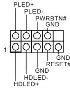
Connect the power button, reset button and system status indicator on the chassis to this header according to the pin assignments below. Note the positive and negative pins before connecting the cables.
