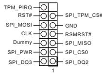
This connector supports SPI Trusted Platform Module (TPM) system, which can securely store keys, digital certificates, passwords, and data. A TPM system also helps enhance network security, protects digital identities, and ensures platform integrity.
