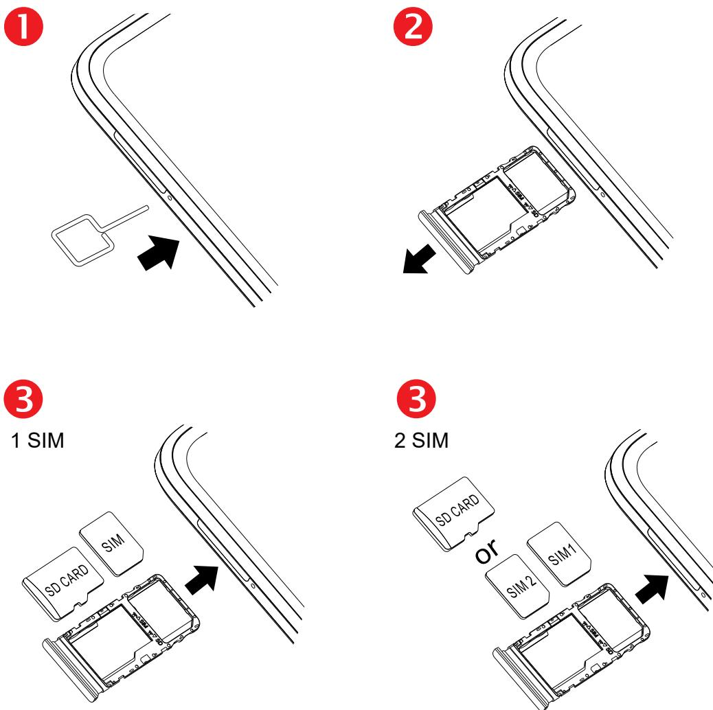
You must insert your SIM card to make phone calls. You do not need to power off your phone before inserting or removing the SIM card as this phone supports hot swap.
