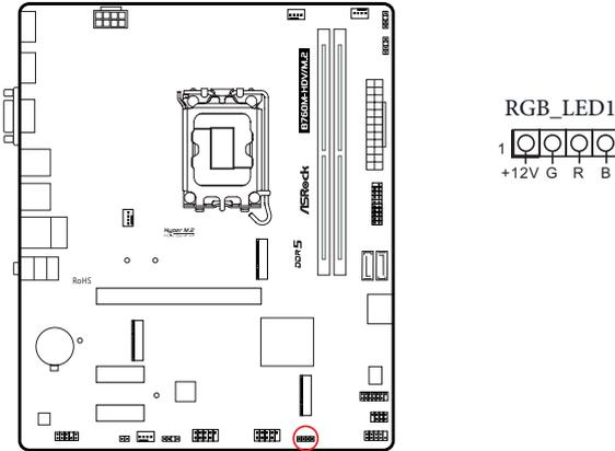
Connect your RGB LED strip to the **RGB LED Header (RGB\_LED1)** on the motherboard.
