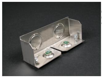
Closes off open end of S4000 Base. Use when end feeds are required for an installation. Includes two 1/2'' - 3/4'' trade size KOs and two No. 10-32 ground terminals.
