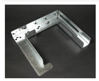
Suspends S4000, 4000, or 6000 Series Raceway from structural ceiling. Designed for use with 3/8" (9.5mm) rod. Hangers should be installed no more than 5' (1.5m) apart along raceway run. Can be bolted back-to-back for dual runs of 3000, 4000, or 6000 Series Raceway.
