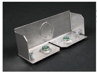
Closes off open end of S4000 Base. Use where one end feed is required in an undivided installation. Includes one 1/2'' - 3/4'' trade size KO and two No. 10-32 ground terminals.
