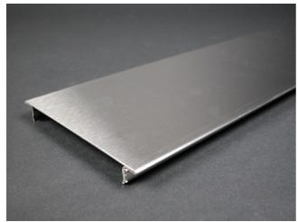
.040" (1.0mm) stainless steel. Snap-on cover for mounting 9" (229mm) device plates on 24" (610mm) centers. Precut to 19.5" (495mm).
