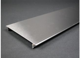
.040'' (1.0mm) stainless steel. Snap-on cover for mounting 9'' (229mm) device plates on 24'' (610mm) centers.
