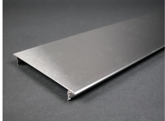
.040" (1.0mm) stainless steel. Snap-on cover for mounting 4 1/2" (114mm) device plates on 18" (457mm) centers.
