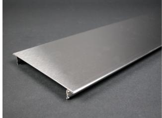
.040" (1.0mm) stainless steel. Snap-on cover for mounting 4 1/2" (114mm) device plates on 12" (305mm) centers.
