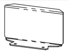
Used to close off unused gangs. NOTE: For use with RFB4E, RFB6 and RFB6E Series Floor Boxes.
