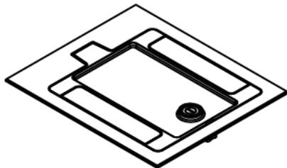
The RFB9 and RFB11 Series Carpet Cover Assembly is a flush with floor, cast aluminum cover assembly with a carpet cutout area, available in powder coated black finish. Maximum load capacity 3,000 lbs. UL Listed to U.S. and Canadian safety standards to meet UL requirements under UL514A for scrub water exclusion. NOTE: Not for use on bare concrete floor applications.
