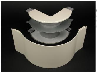
Full capacity 90 degree external corner. Used in both divided and undivided applications. Provides 2" (51mm) cable bend radius control for UTP, STP and fiber optic installations. Ideal for new installations whether the cable is lay-in or pull-through.
