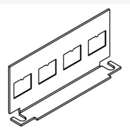
Communication bracket with four (4) RJ opening knockouts. Use as blank plate or for up to four RJ openings. Opening dimension is 9/16" x 3/4" [14.3mm x 19.1mm]. NOTE: For use with RFB4-Cl-1 only.
