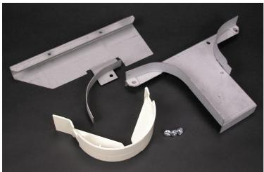
Radiused insert for the 4015D Divided Tee. Provides 2" (51mm) cable bend radius control for UTP, STP and fiber optic cable installations. Ideal for new or retrofit applications whether cable installation is lay-in or pull-through.
