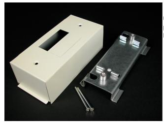
Cover used as is with single-pole breaker. KO is removed for twopole. For two-pole circuit breakers where the toggle is center located, web is snipped or cut out.
