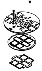
Nonmetallic slide holder assembly. Available in black (BK), gray (GY), ivory (VY), nonmetallic brass (BS), and nonmetallic aluminum (AA). Assembled with scrub water gasket. For use on tile or carpet floors.
