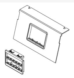
For AC8850 Box. Includes one (1) Ortronics Series II and one (1) TracJack adapter. NOTE: AC8850 is a single-service box. Power plates cannot be used in conjunction with communication plates.
