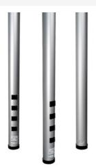
Satin anodized extruded aluminum pole. Nominal material thickness .060" (1.5mm). Length: 10' 5" (3.2m). Two-compartment (power and communication channels). Factory wired with four 15A 125V NEMA 5-15R devices. Provided with one 1/2" [12.7mm] trade size KO in cover at base for communications. T-bar mounting hardware, ceiling trim kit, and feed box furnished. NOTE: There is no method provided for mounting data in this pole.
