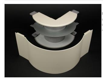
Full capacity 90 degree external corner. Used in both divided and undivided applications. Provides 2'' (51mm) cable bend radius control for UTP, STP and fiber optic installations. Ideal for new installations whether the cable is lay-in or pull-through.
