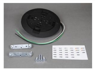
Quad 15A receptacle included for standard or isolated ground wiring. Unit complete with link straps, adapter plate and receptacle bracket to attach preset or afterset.
