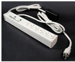
Perma Power computer grade surge protection. Six outlets, remote switch, durable putty white aluminum housing, 15A. 15' (4.6m) 14/3 SJT putty white cord with NEMA5-15 plug. Length 13 1/4"" (337mm). Snap-on, slide-off mounting.
