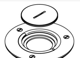
Brass communications or power cover plate with 2 1/4" (57mm) threaded opening for tile. NOTE: For carpet or tile installations. All cover plates are furnished with gasket and three screws. The 895P Polycarbonate Series Cover Plates must be field modified for dual service.
