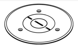
Polycarbonate communications or power cover plate. Includes one plug with 3/4" (19mm) opening, one plug with 1" (25mm) opening, and one plug with 2 5/8" (67mm) opening. For pass-through only. NOTE: For carpet or tile installations. All cover plates are furnished with gasket and three screws. The 895P Polycarbonate Series Cover Plates must be field modified for dual service.
