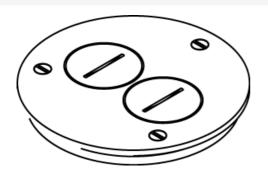
Brushed aluminum cover plate with two screw plug openings, 4 1/4" (108mm) for tile. NOTE: For tile installations. All cover plates are furnished with gasket and three screws. The 895P Polycarbonate Series Cover Plates must be field modified for dual service.
