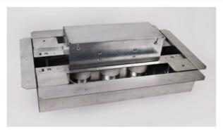
3-Gang Fire Classified Steel Floor Box. Adjustment range over deck of 2" (51mm) minimum to 5" (127mm) maximum. Three 1 1/4" (32mm) conduit feed openings. Inside Gang Capacity - 67.5 cubic inches. Outside Gang Capacity - 54 cubic inches each gang. This floor box preserves the 2-hour fire rating of floors in which it has been installed.
